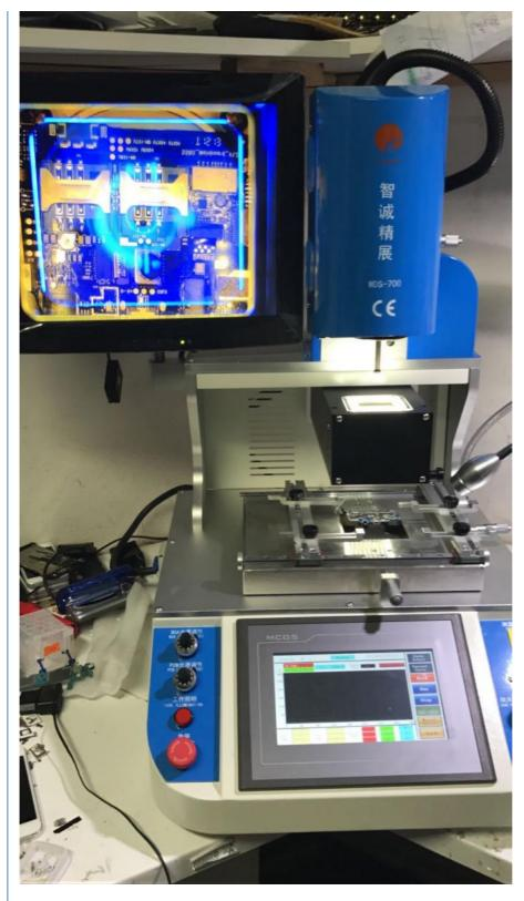
**Multi-functional and humanized operation system** 1.Adopting the HD touch human-machine interface;upper heating head and mounting head designed 2 in 1;providing many kinds of titanium alloy BGA tuyere can be rotated in 360 degree for easy installation and replacement. 2.X,Y and R angle adopted micrometer fine-tuning,accuracy locating,precision can reach ±0.01mm.
