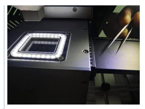
4. Auto feed chip, auto pick up chip, auto blowing chip, can identify the central position automatically when optical alignment;
