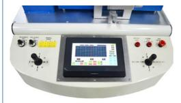
6.Uses the high precision K-type thermocouple closed-loop control which is imported from USA,with the unique heating method, ensure the weld temp precision control within  $\pm 1$  °C
