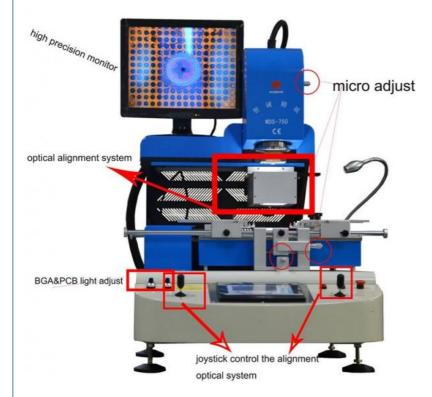
3.3 independent heating zones, each heating zone can set up the heating temp, heating time, temp rise rate; Six period of heating temperature, simulate the reflow heating mode, set up as Preheating, keeping, heating, welding, welding, cooling;
