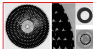
Due to the X-ray (2D imaging) detection principle, stacked or non-tiled materials cannot be counted. Currently, for the entire industry, materials such as ultracaps cannot be accurately counted by the X-ray counting machine.
