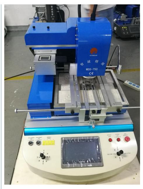
10. Equipped the extra camera to obverse the solder ball melting, to ensure the temp curve and weld effect(this function is optional).
