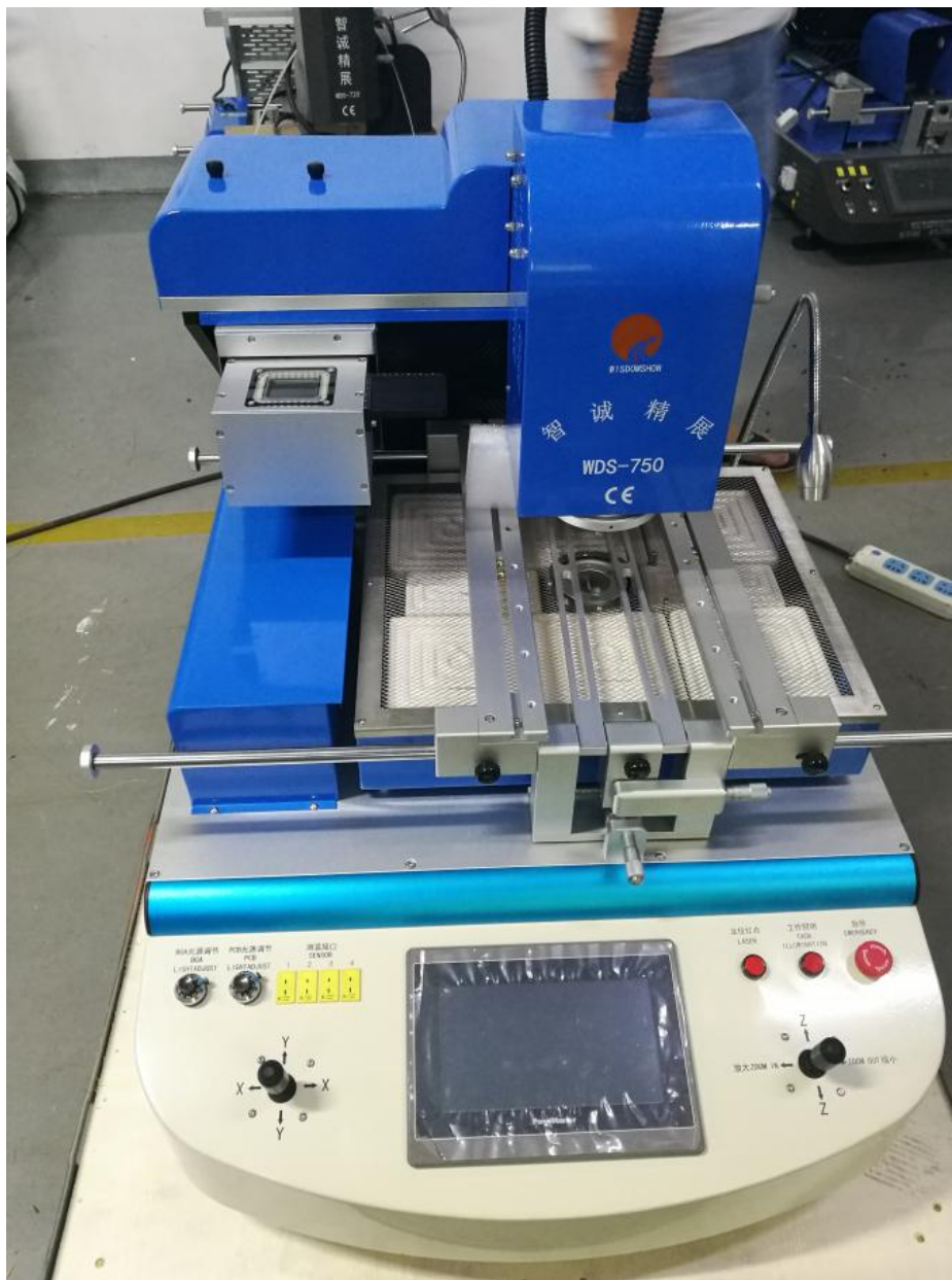
10. Equipped the extra camera to observe the solder ball melting, to ensure the temp curve and weld effect (this function is optional).
