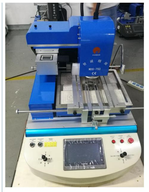
10. Equipped the extra camera to obverse the solder ball melting, to ensure the temp curve and weld effect (this function is optional).
