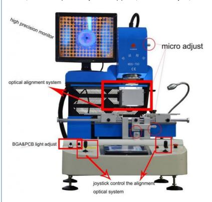
3.3 independent heating zones, each heating zone can set up the heating temp, heating time, temp rise rate; Six period of heating temperature, simulate the reflow heating mode, set up as Preheating, keeping, heating, welding, welding, cooling;
